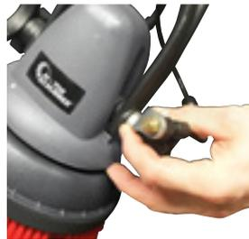
3. Screw the locking knob back into position, clockwise.
